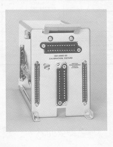
The 067-0590-00 Plug-In Extender is designed primarily for use with the Tektronix Type 568 or R568 Oscilloscope when calibrating or troubleshooting the Type 3S5 or 3S6 Programmable Vertical. The Extender can also be used with the Type 568 or other 560-Series Oscilloscopes to extend digital vertical plug-in units, as well as non-digital vertical and time-base units.
